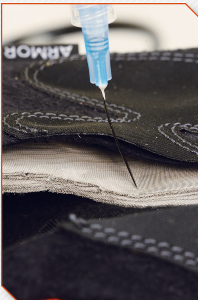
25 gauge needle buckling
