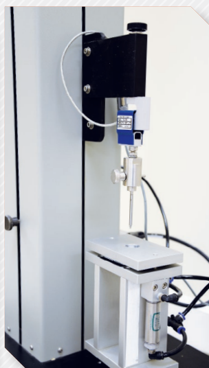
EN388:2003, 6.4 Puncture Test
