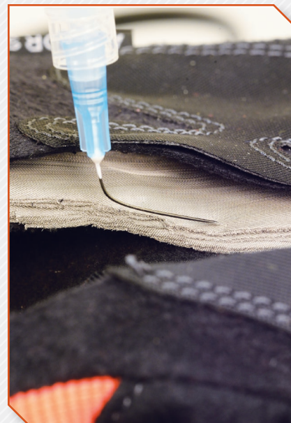
25 gauge needle failure
