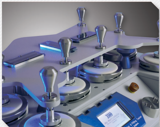
EN388:2003, 6.1 Abrasion Test
